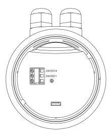
1 X 24VDC+ \_\_\_24VDC 3 X ⊕ \_\_\_ GND
