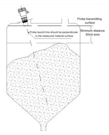
Installed on container flange
