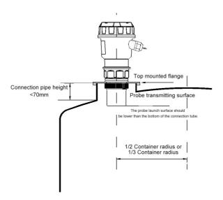
Installed on flange-dome roof
