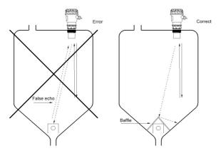
A projection with a flat top at the bottom of the container-a refracting plate should be added.
