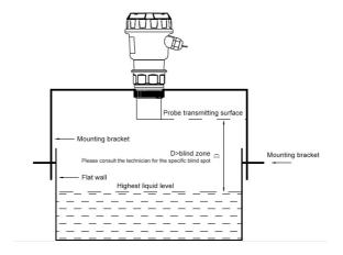
On Open tank -Top Center Bracket Installation
