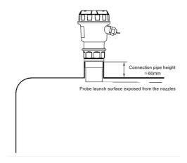
The probe is mounted on the threaded nozzle.
