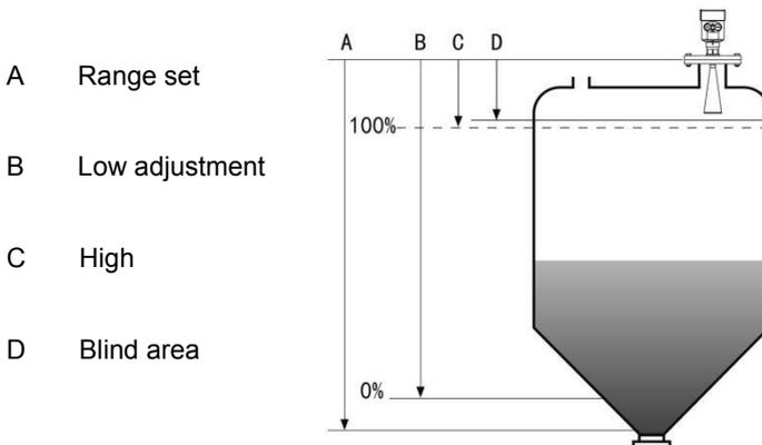
**Datum measurement:** Screw thread bottom or the sealing surface of the flange.
