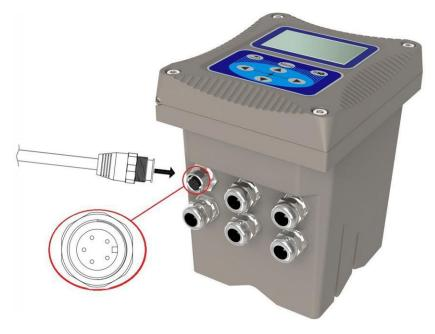
Figure 10 The Diagram of Sensor connection
