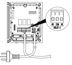
Figure 9 Relay Wiring
