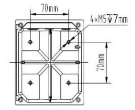
Figure 3 Installation Size
