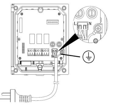
Figure 8 Power Supply Wiring
