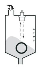
The transducer should not be mounted too close to the tank wall, the build-up on the tank wall cause false echoes.
